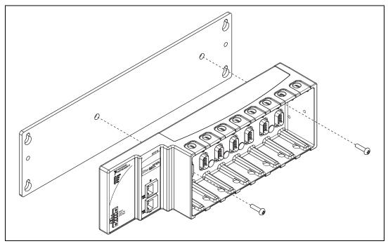
Figure 5. Installing the Panel Mount Accessory on the NI 9144 Chassis
